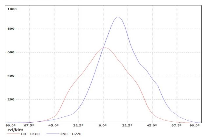
Luminaire: Ledil Oy CN13169\_LENA-WAS-DL (Cree CXA20 698Im @ 250mA) Efficiency=75% Lamps: 1 x Cree CXA20 698Im @ 250mA
