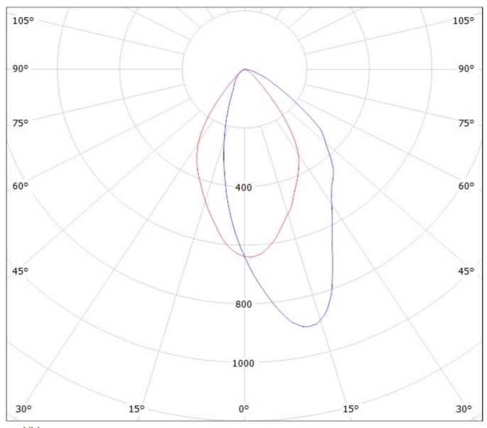
cd/klm \_\_\_\_\_\_ C0 - C180 \_\_\_\_\_ C90 - C270 NOTE: The typical divergence will be changed by different color, chip size and chip position tolerance. The typical total divergence is the full angle measured where the luminous intensity is half of the peak value.
